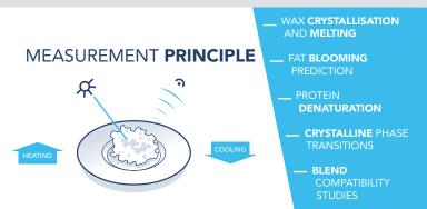
Rheolaser Crystal uses the Diffusing Wave Spectroscopy principle (DWS). Light is scattered by the particles, creating an interference pattern (Speckle Image). The variation of this image is directly related to the motion of the particles: the faster they move, the faster the Speckle Image changes. By a mathematical analysis of this variation, decorrelation functions can be computed and then processed, to obtain a characteristic time  $\tau$ , as a function of time or temperature.
